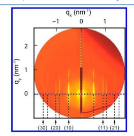
**Figure 2.** In situ SAXS pattern of a ML of 11.8 nm diameter NPs. The separation of cores is fit by the first five peaks: (1 0), (1 1), (2 0), (2 1), and (3 0).
