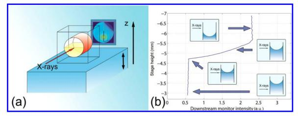
Figure 1. (a) Schematic showing the SAXS setup. (b) Alignment of the horizontal X-ray beam with the horizontal liquid surface for grazing incidence SAXS (GISAXS), by downstream monitoring of the transmitted X-ray beam as the cell is translated. Measurements are performed in the configuration of the inset with the dashed line path.
