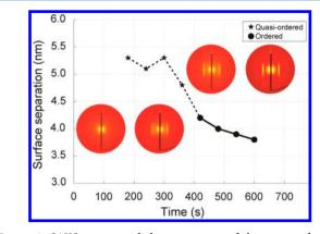
**Figure 4.** SAXS images and the separations of the core surfaces of nearest-neighbor iron oxide NPs during the formation of a hexagonally ordered array, along with representative SAXS images, after drop-casting 13.2 nm NPs in heptane. The formation of quasi-ordered MLs begins at ~180 s, followed by fully ordered ML starting at ~420 s.
